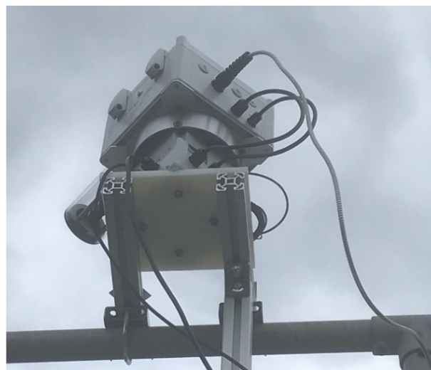
Our new MAX-DOAS instrument up and running on the Torrington Place rooftop at UCL
