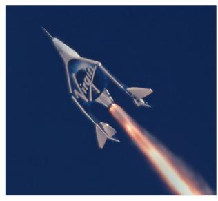
Hybrid: solid fuel (HTPB) + liquid oxidizer (N<sub>2</sub>O)
